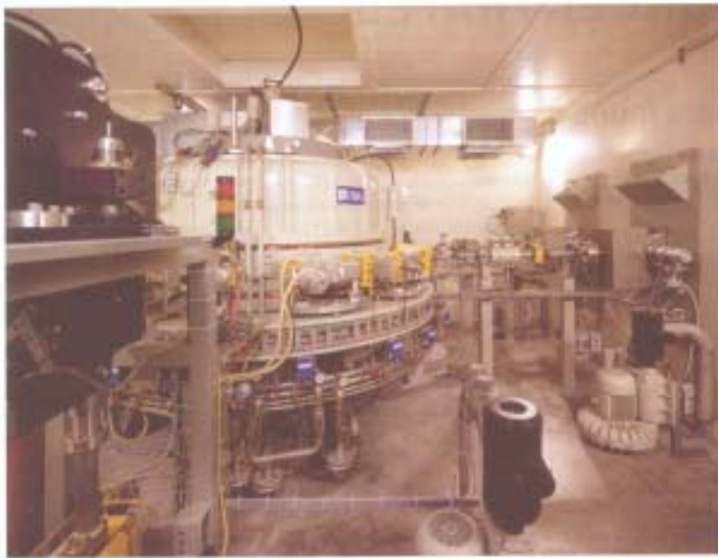
DE-BUGGING IBA facility in Bridgeport, N.J., sanitizes mail headed for Washington, D.C., using electron-beam irradiation.
