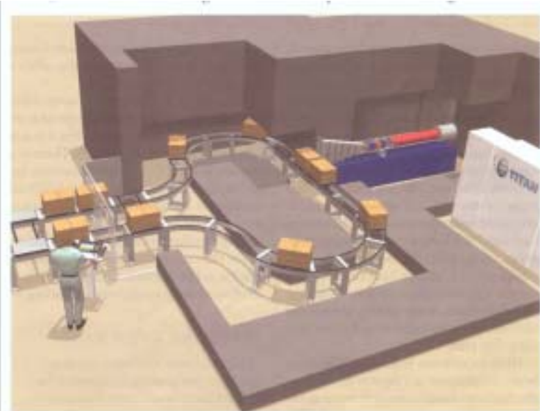
SAFE PASSAGE Boxed mail travels along conveyer system to an electron beam where high-energy electrons destroy anthrax and other biohazards.
